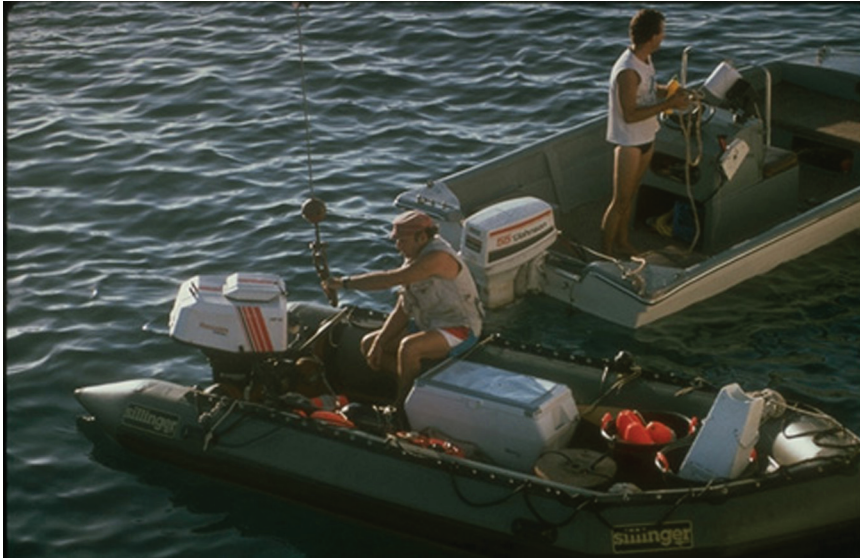
Figure 4. The electronic remote survey tender preparing to launch. To protect it from the sea, the magnetometer is in the white chest. Note also the buoys.
